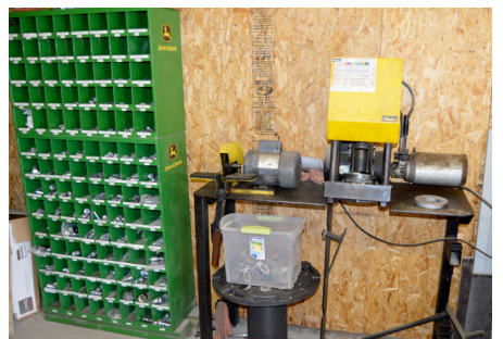
HYDRAULIC HOSE SETUP W/ FITTINGS AND PRESS
