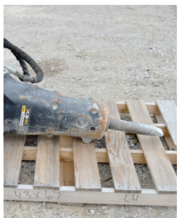
SKID LOADER JACK HAMMER
